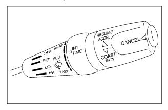
Use this lever located on the right side of the steering wheel to operate the windshield wipers and washers.
